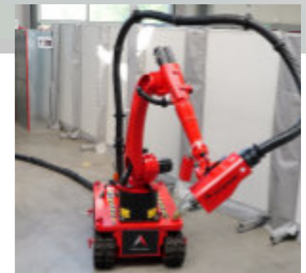
Large mobile working area thanks to a 15 m long energy chain.
