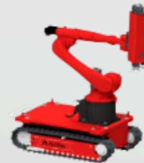
6-axis robot and crawler track with remote control
